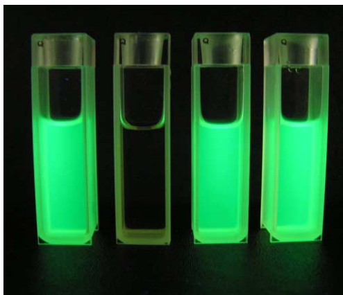
Figure 3. Fluorescence of 3 in the absence and presence of metal ions. From left to right: no metal ion, in the presence of \text{Ca}^{2+} , \text{Mg}^{2+} , and \text{K}^+ ions. [3] = 2.5 \times 10^{-6} M and [M^{n+}] = 1.25 \times 10^{-4} M in MeOH- \text{H}_2\text{O} (95:5, v/v).
